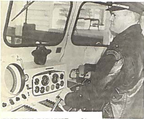
CAPTAIN'S PARADISE — Lieutenant John Younger steers the Intrepid down river while scanning the ultra-modern control panel which includes depth sounding gear for shallow water and radar for "shallow visibility."
